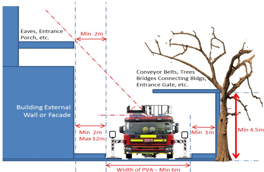
**Figure 3b. Overhead and lateral clearance for Fire Appliance Accessway**
