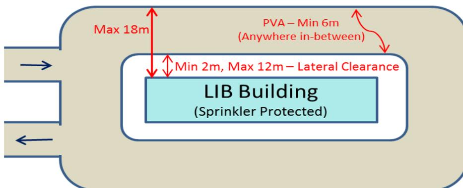
Where the LIB is not sprinkler protected, DFES believes that a minimum distance of 10 metres should exist between the subject structures (LIB) and the near side of the PVA. Detailed explanation is available on the DFES website in 'Technical Note 03/16 Perimeter Vehicular Access – Large Isolated Buildings'.
