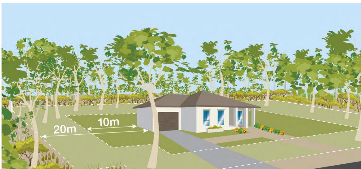
**Figure 5:** Measuring zones around a building
