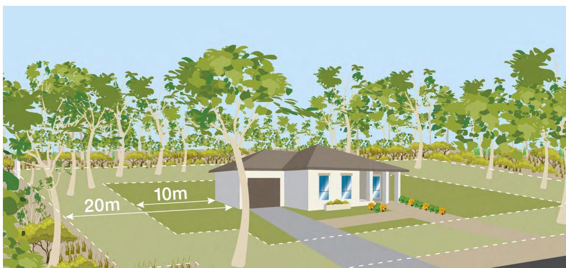
**Figure 5: Measuring zones around a building**
